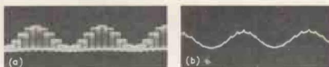
Fig. 4(a). Sine wave circuit—no smoothing (b). Sine wave circuit—0.05μF smoothing
