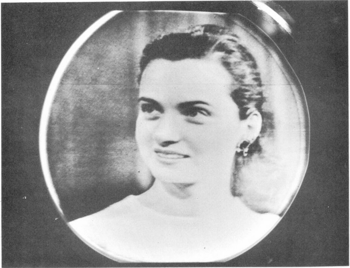
Figure 7. One field of a television picture stored on a 5-inch Tonotron tube
