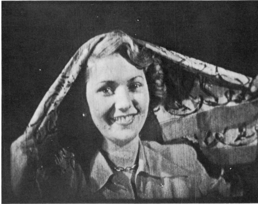
Fig. 13 - Photograph of a half tone color slide transmitted by the Tricolor Vidicon and displayed as in Fig. 11.
