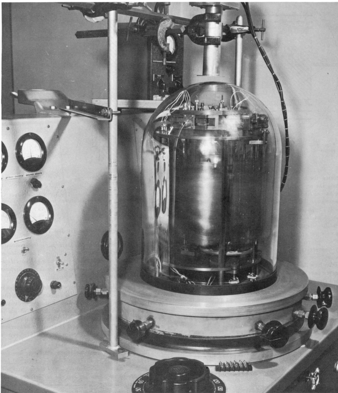
Fig. 7 - View of an evaporation system with the precision jig in place for making Tricolor Vidicon targets.
