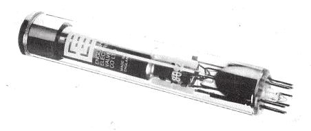
The range of spectral sensitivity of the P8092 is determined by the transparency of its window. The germanium faceplate is bloomed to give optimum sensitivity in the 8 to 14 micron band in which there is maximum radiant power from objects at temperatures close to ambient.
