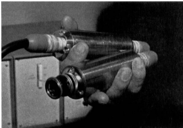
FIG. 7. Miniaturized camera employing \frac{1}{2} -in. vidicon for internal examination of pipes.
