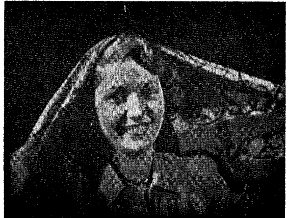
Fig. 10—Photograph of a color picture transmitted by a developmental tricolor vidicon. Three output signals were added together and displayed on a black-and-white monitor. The streaks are not inherent, but arise from nonuniformity in the evaporation grill used in fabricating the target.
