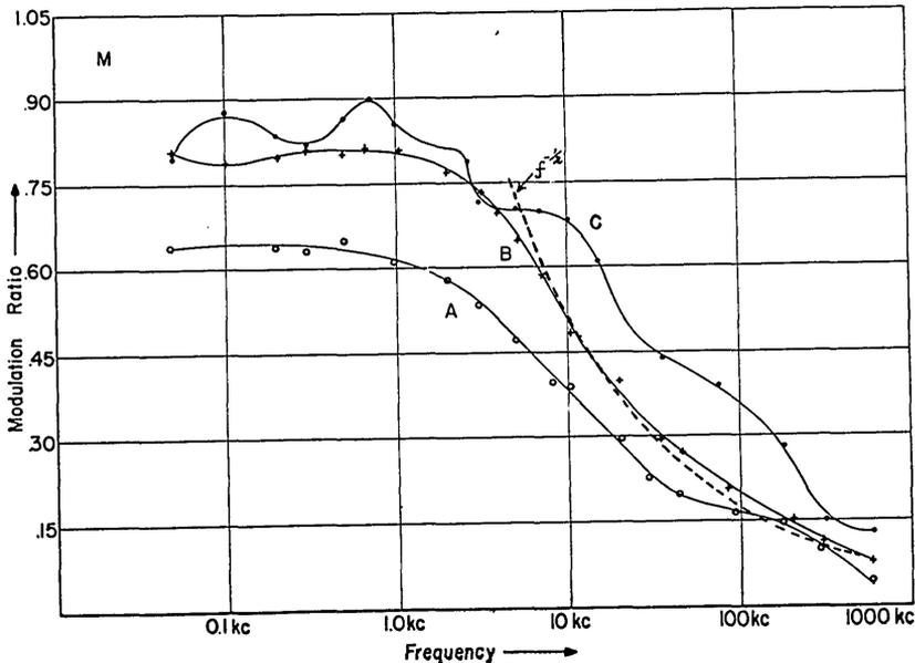
FIG. 7. Radiation-current modulation ratios for three lamps. The dashed curve in the case of lamp B shows how the ratio would vary if it is assumed that it is inversely proportional to the square root of the frequency.
