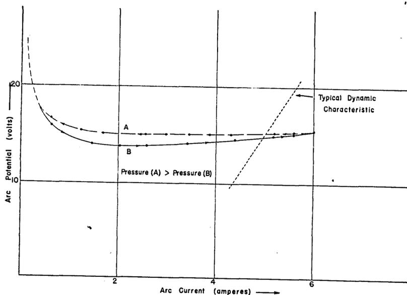
between readings a single curve is obtained. A typical dynamic characteristic is also shown.
