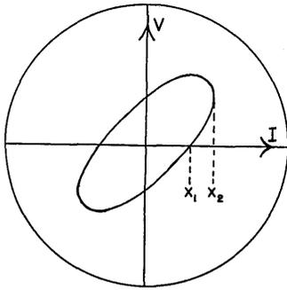
FIG. 4.  $\sin\theta = x_1/x_2$ ,  $\theta =$ angle between current and potential waves.
