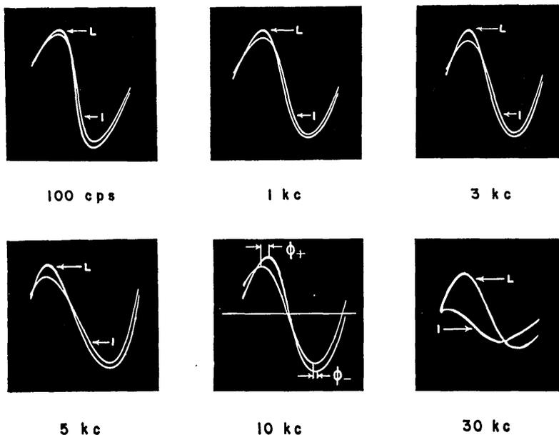
FIG. 9. Photographs of oscilloscope traces of superimposed current and light waves for several modulation frequencies.
