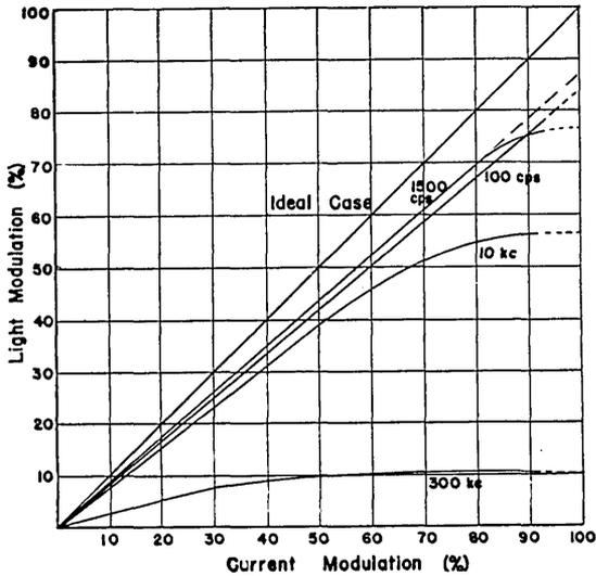
FIG. 6. Variation of observed percent light modulation with depth of current modulation at several frequencies.
