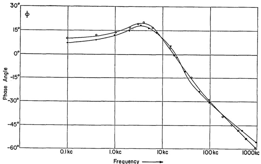
FIG. 5. Measured angle of lag of current behind potential plotted as a function of the modulation frequency.
