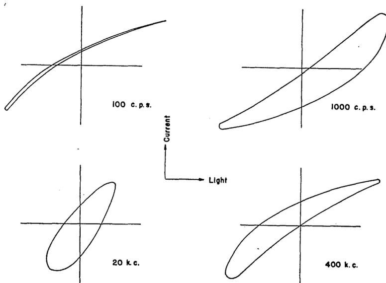
FIG. 8. Typical oscillograms obtained when the current and light waves are applied to the vertical and horizontal sweeps of the oscilloscope.
