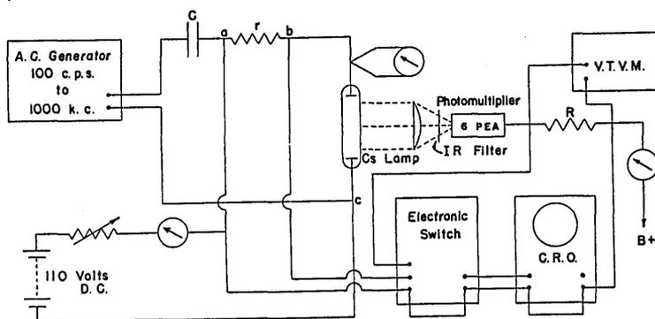
FIG. 3. Block diagram showing all components of the measuring circuit.
