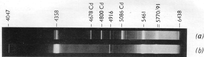
Fig. 14.—Spectra of Osira H.P.M.V. Fluorescent Lamps. (a) 400w. H.P.M.V. Fluorescent Lamp. (b) 80w. and 125w. H.P.M.V. Fluorescent Lamps. (Wavelengths in Angström Units).
