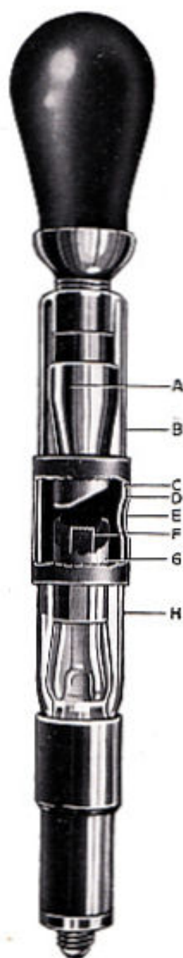
Figure 1. —A heavy Anode insert tube for the "METALIX" Universal Shockproof Shield. Cooling is effected by thermal storage in a solid metal body specially shaped to conform with the electric field, and having a blackened surface from which the heat is continuously dissipated by radiation. In the illustration, part of the centre of the tube is cut away to show its internal arrangement.
