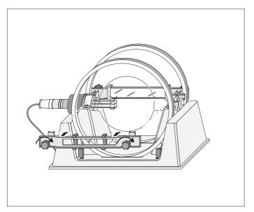
Attach the straight member with mirror horizontally to the back Helmholtz coil and the member with two slides to the front Helmholtz coil.
