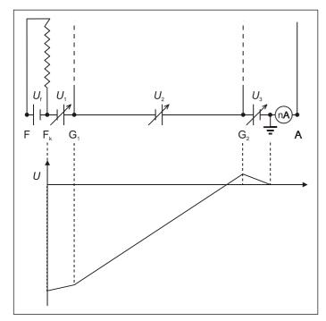
Cathode heating:  $U_{\rm f}$  = 6.3 V AC/ DC, floating Emitting grid voltage:  $U_1 = 0 \dots 5.0 \text{ V DC}$ , floating Accelerating voltage:  $U_2 = 0 \dots 30.0 \text{ V DC}$ , floating Countervoltage:  $U_3 = 0 \dots 5.0 \text{ V DC}$ , floating
