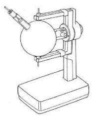
**h** Switch on the coils circuit. Use the rheostat to steadily increase the current. The spot on the screen should be deflected more and more as the current in the coils increases.
