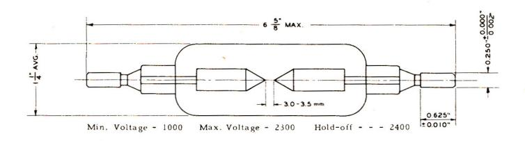
This flashtube has an arc length of only 3.0 to 3.5 mm. The shape of the arc is approximately spherical, with a diameter of about 12 mm at the maximum loading. This small size is important in many optical devices which can utilize light from only limited areas.
