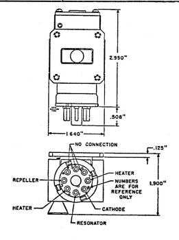
Reflex klystron having a B8-21 small wafer octal 8 pin base, and provision for manual tuning.
