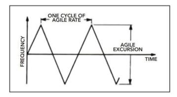
Agile Excursion: The total frequency variation of the transmitter during agile operation.
