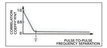
Using this relationship, one finds that a radar operating at a 0.5  $\mu$ s pulse duration will have efficient decorrelation between target echoes if pulses differ in frequency by at least 2 MHz. Note that the required frequency separation is a function only of the pulse duration.
