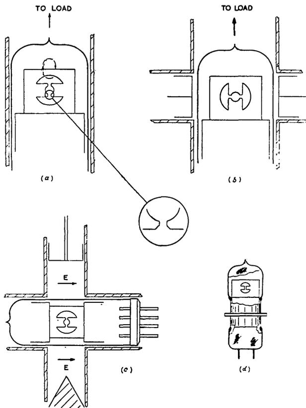
Fig. 6.—Arrangements of 2-segment symmetrical anode.
