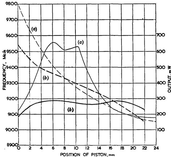
Fig. 16.—Tuning characteristics of 2-segment s.a. valve.
