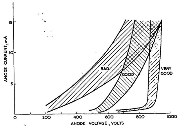
Fig. 7.—Cut-off characteristics for  $H = 2400$  oersteds.
