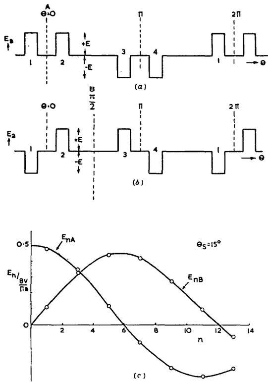
Fig. 4.—Field distribution and component amplitudes for  $\pi/2$  mode (m.s.).
