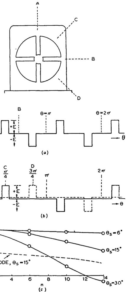
Fig. 5.—Field distribution and component amplitudes for  $\pi$  and  $\pi/2$  modes (s.a.).
