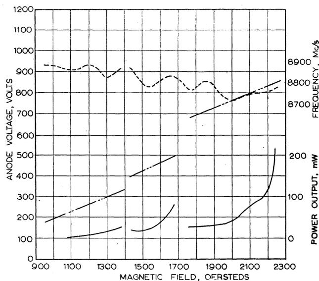
Fig. 8.—Performance of 4-segment m.s. valve.
