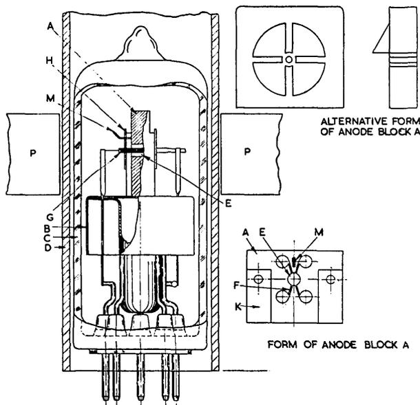
Fig. 1.—General arrangement of spatial-harmonic valve.
