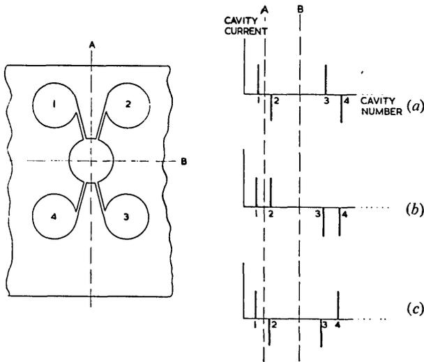
Fig. 2.—Distribution of current in m.s. anode.
