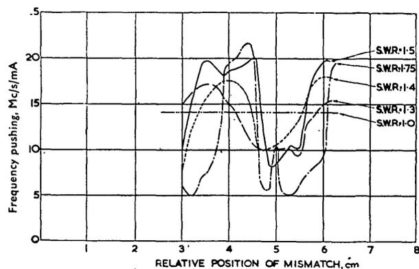
Fig. 14.—Variation of frequency pushing with circuit loading.
