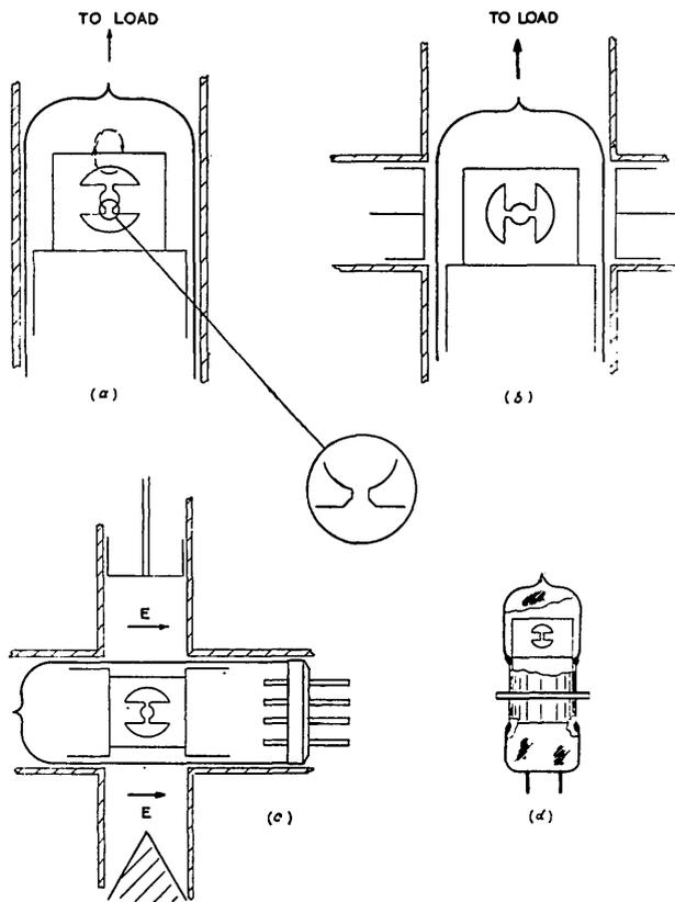
Fig. 6.—Arrangements of 2-segment symmetrical anode.
