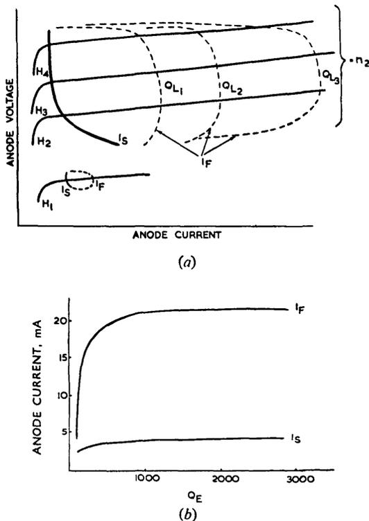
Fig. 13.—Influence of load coupling on  $I_S$  and  $I_F$ .
