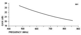
Fig. 1. IOTD250 typical gain characteristic
