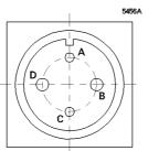
Pins A and C are connected within the circuit assembly for use as an interlock circuit; this connection may be removed by the customer if required for other purposes, but the loss of interlock should be borne in mind.
