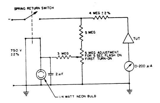
FIGURE 4. Ignitor discharge circuit.
