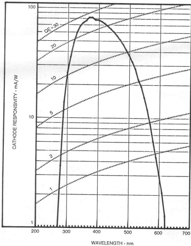
**Figure 1 - Typical Photocathode Spectral Response Characteristic**
