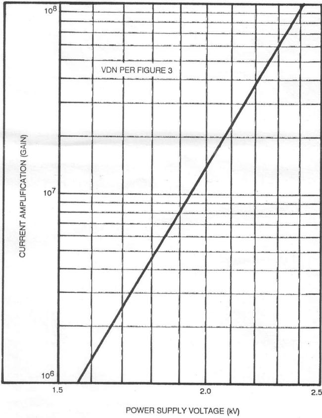
Figure 5 - Typical Current Amplification Characteristic
