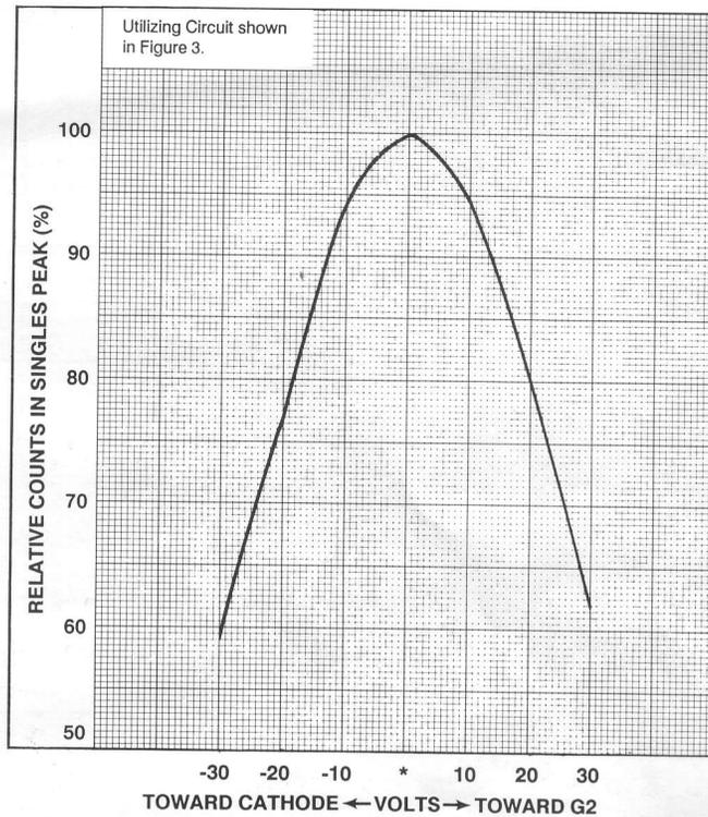
**Figure 2 - Typical Effect of Grid No.1 Potential Variation on Count Rate**
