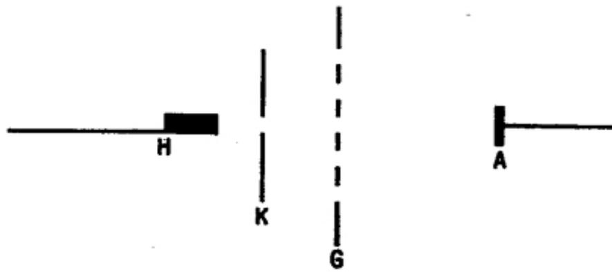
Fig. 4.1. The electrode structure of the glow thyatron.
