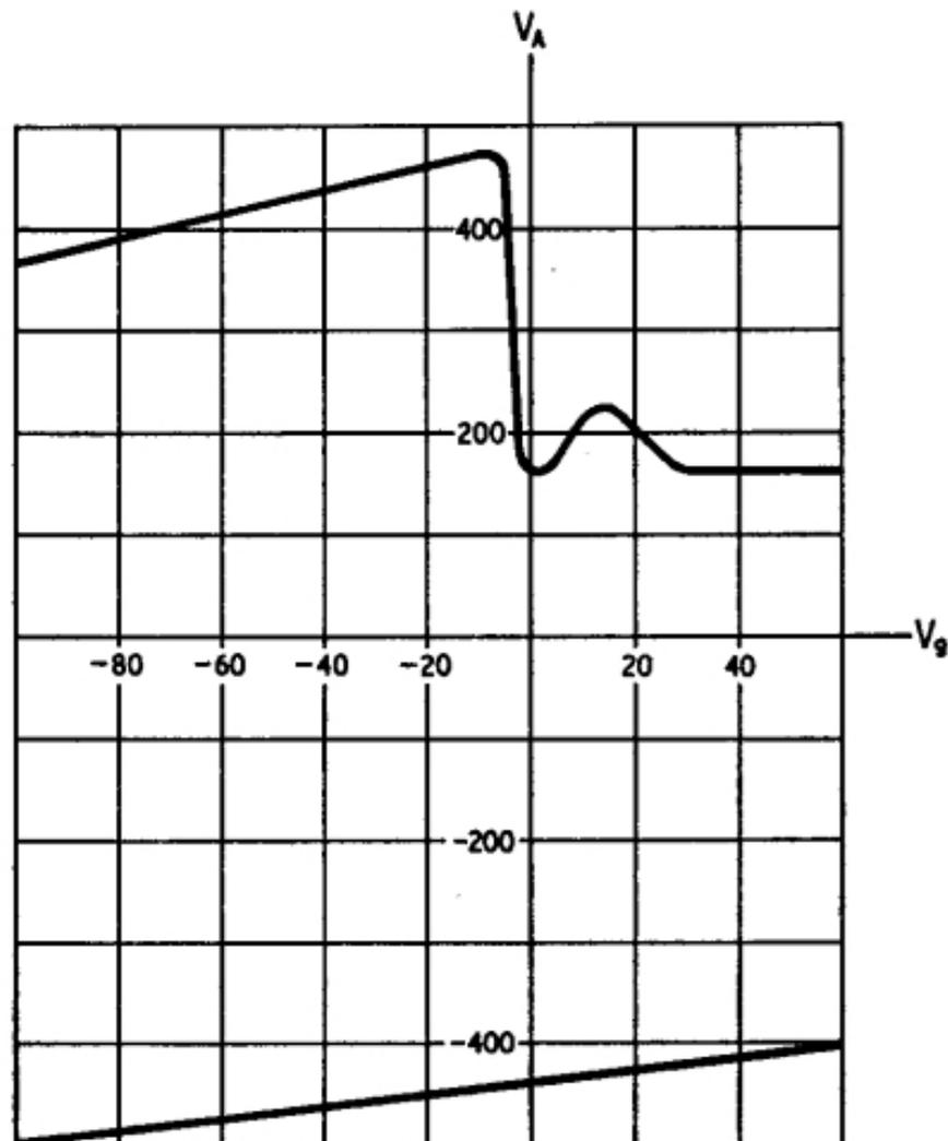
Fig. 4.2. The glow thyatron firing characteristic.
