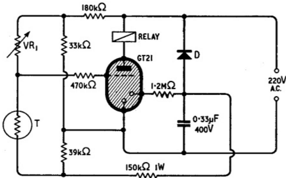
Fig. 4.4. A thermostat circuit.
