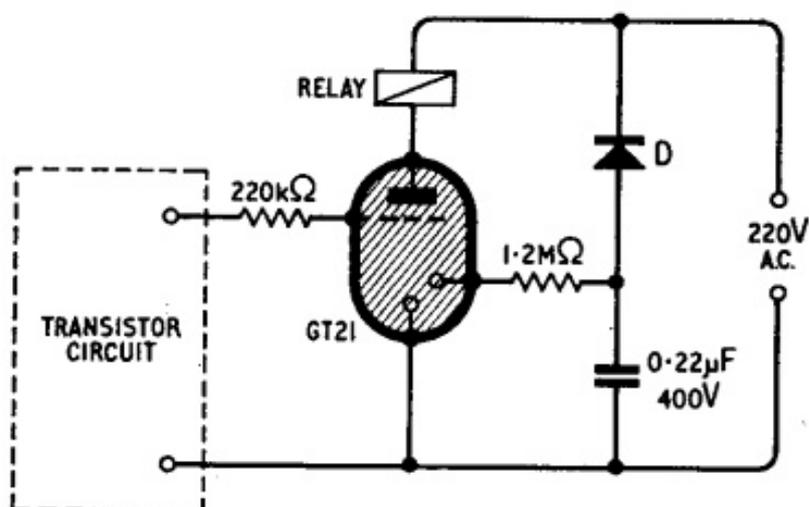
Fig. 4.5. Control of a glow thyratron by a transistor circuit.
