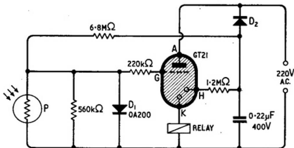
Fig. 4.3. A circuit for controlling a relay by a light beam.
