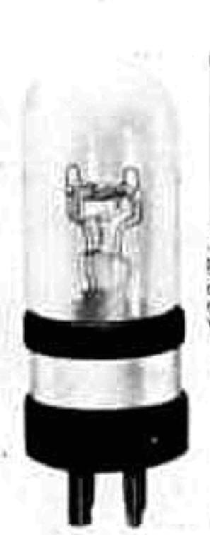
For old style L. F. amplifiers EV 89 a, b, c, EV 132 and EV 176. / Straight filament and iron resistance, heating current 0,53 to 0,56 amps., anode voltage 90.
