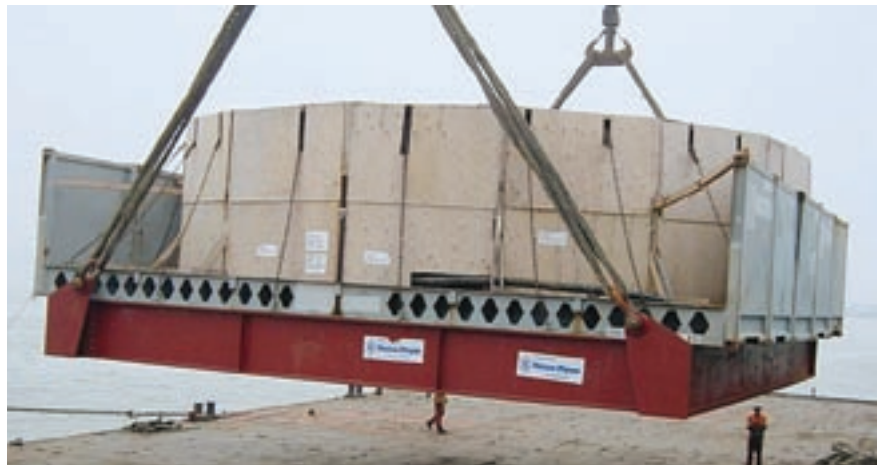
Loading of a steel pallet containing 500 tons of submarine cables for China
