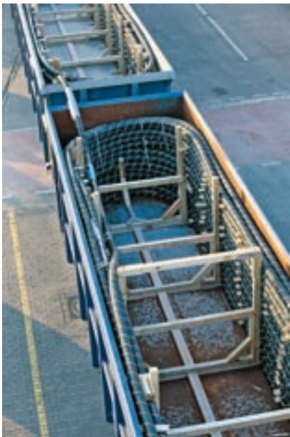
Transport of a submarine cable in a railcar unit
