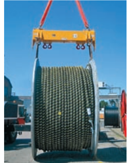
Lifting a submarine power cable drum
