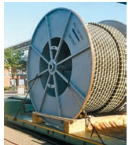
Transport of a submarine cable drum on a heavy load trailer
