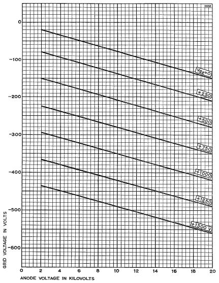
The above graph is for an average tube. To allow for variations between tubes and to cover changes during life the working bias voltage shown on the graph should be exceeded by at least 20% (see note 8 on page 3).
