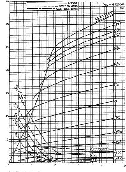
ANODE VOLTAGE IN KILOVOLTS
