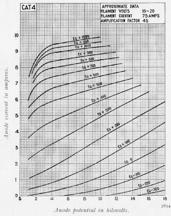
Taken at filament volts to give 10 amperes emission at 90 per cent. saturation.
