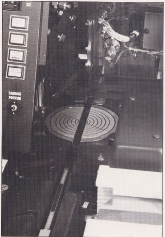
Automatic wafer loading system
