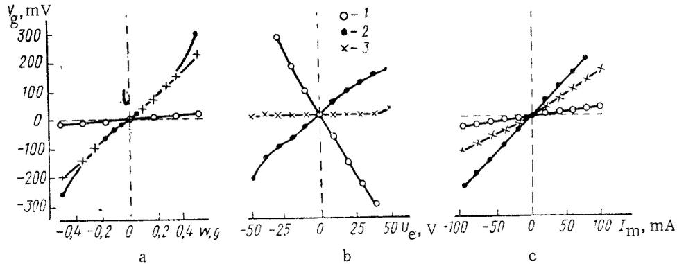
Fig. 6. Static displacement characteristics of the charge in the following fields: a) gravitational; b) electric; c) magnetic. Discharge current  $i_c$  denoted as 1 = 0.3, as 2 = 1.7, and 3 = 1.1 mA.
