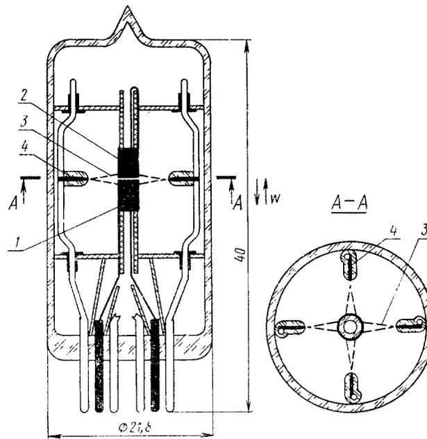
Fig. 13. Inplatron with the cylindrical anodes 2 and 1, four gas-discharge columns 3, and the cathodes 4.
