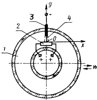
Fig. 12. Inplatron with the toroidal bulb 1 and the film resistance 2 which forms the anode; 3) cathode and 4) gas-discharge column.
