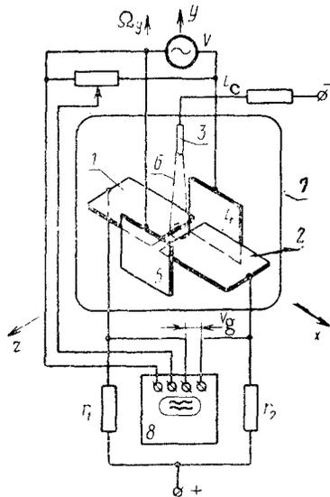
Fig. 7. Schematic of the equipment for observing the gyroscopic effect: 1, 2) differential anodes; 3) cathodes; 4, 5) z-transverse electrodes; 6) gas-discharge column; 7) bulb; 8) double-beam electronic oscillograph.
