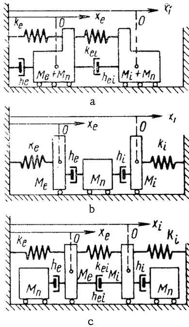
Fig. 8. Mechanical models of the "discharge - electrode - external circuit" oscillatory system:  $x_e$  and  $x_i$  are coordinates;  $k_e$ ,  $k_i$ , and  $k_{ei}$  are quasi-elasticity factors;  $h_e$ ,  $h_i$ , and  $h_{ei}$  are resistance factors;  $M_e$ ,  $M_i$ , and  $M_n$  are the effective masses related to the partial systems of the envelope  $e$ , the core  $i$ , and the medium  $n$ .
