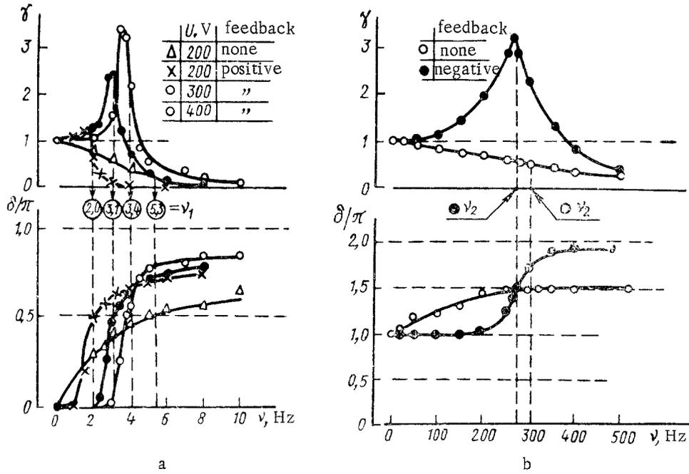
Fig. 5. Amplitude-frequency and phase-frequency characteristics: a) positive velocity feedback and inertial excitation;  $i_c = 1.6$  mA; amplification factor of  $10^3$ ;  $C_{sh} = C = 0.1$   $\mu$ F;  $R = 100$  k $\Omega$ ; b) negative velocity feedback and electrical excitation;  $i_c = 0.3$  mA; amplification factor of  $10^3$ ;  $C_{sh} = 0$ ;  $C = 0.1$   $\mu$ F;  $R = 13.8$  k $\Omega$ ;  $U_b = 200$  V.
