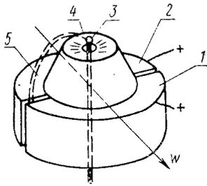
Fig. 10. Hughes' accelerometer: 1, 2) anodes; 3) cathode imbedded in the insulator; 4, 5) gas-discharge column.
