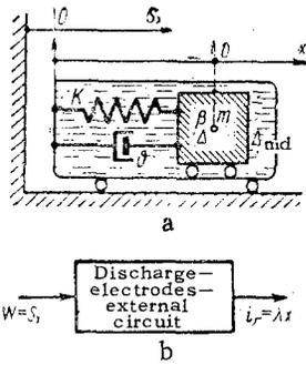
Fig. 9. Electromechanical analog: a) oscillatory system; b) system as a whole considered as a transducer.
