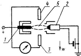
Fig. 11. Stocker and Weston accelerometer: 1) anode; 2) cathode; 3, 4) probe electrodes; 5) gas-discharge column.
