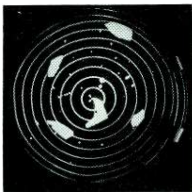
Radar ppi obtained using conical deflection circuit shown in Fig. 7
