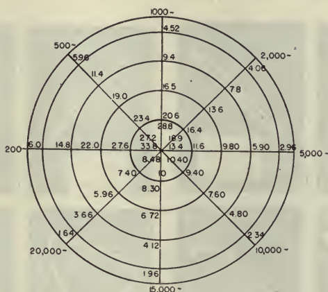
FIG. 11. Relative modulated brightness at various frequencies and at different parts of the light-source spot of a 100-w concentrated-arc lamp.
