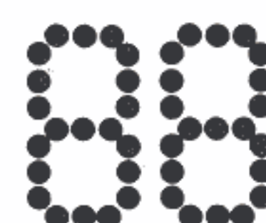
Front View of Double 7-Segment Display
