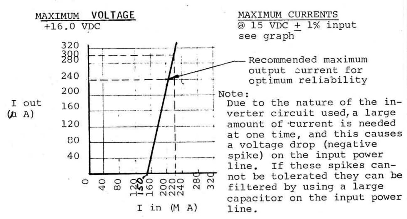
4.1.2 Line Regulation: These power supplies are, in effect, DC transformers. Variations in input voltage are proportionately reflected in output voltage.
