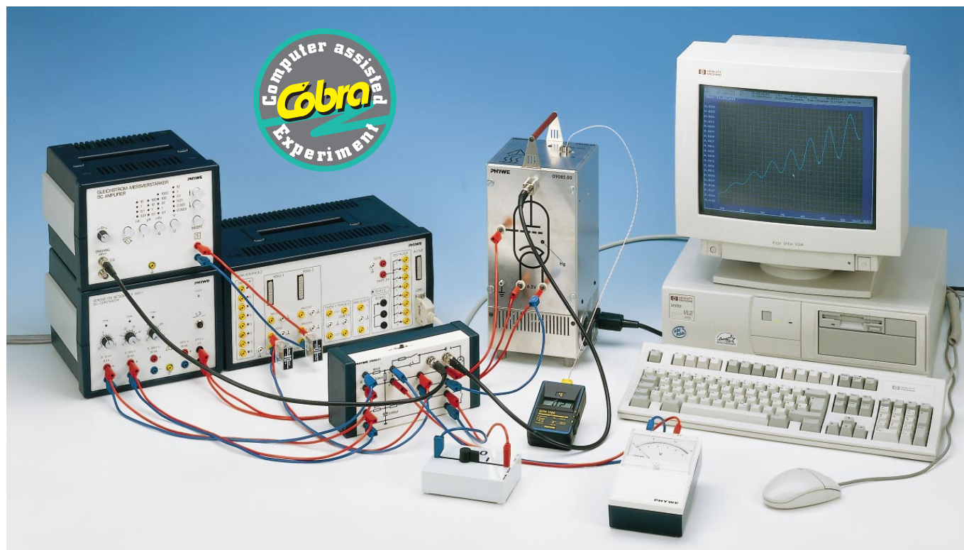
Fig.1: Set-up for the Franck-Hertz experiment with interface.
