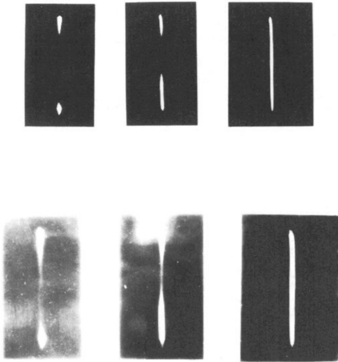
Fig. 2 Initial channel in a \sim 150 pF discharge
