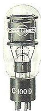
Figure A Max. Over-all Dimensions 5 1/2 x 2 Medium 6 Pin Base
