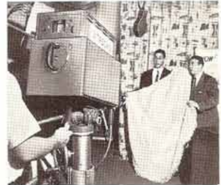
Program in progress. Vitascan mobile camera is used in exactly the same manner as an ordinary camera. Operator focuses and views through electronic viewfinder.
