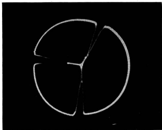
Fig. 7.—Circular trace oscillograph of transmitted signal when 3 out of 30 channels are in operation.
