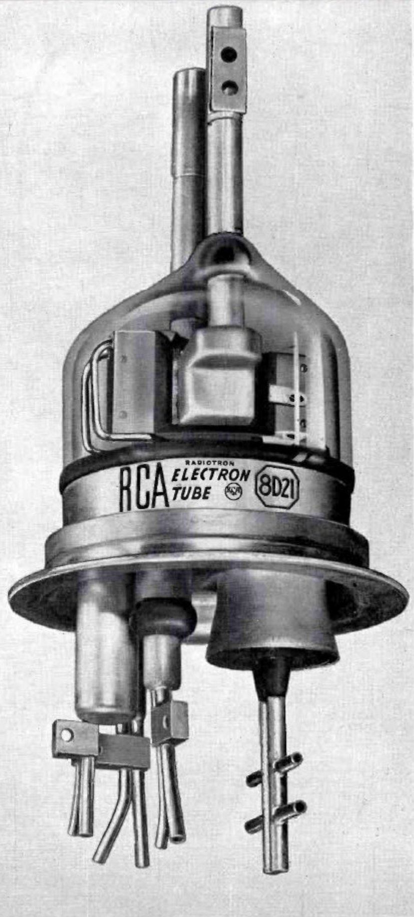
FIG. 2. Finished 8D21 showing how the anode-dome assembly (with anode terminals of tetrodes No. 1 and No. 2 projecting from top) is welded to metal header which supports the internal structure of tube. Directly below metal header and to the right are the control-grid terminals of tetrodes No. 1 and No. 2. To left of center, the terminal for the No. 2 grids; and to the extreme left, the filament terminals. The tube is fitted with a special cathode and beam-confining electrodes, and, because of the cathode structure used, must be operated in a horizontal position with plane of the control grids below horizontal plane of the filament leads.
