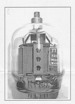
Internally this valve is constructed as two parallel electrode systems in a common anode.
