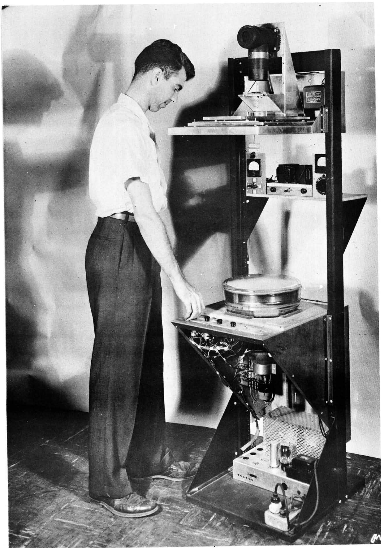
Fig. 7: Optical Test Stand To Check Deflection-Circularity.
