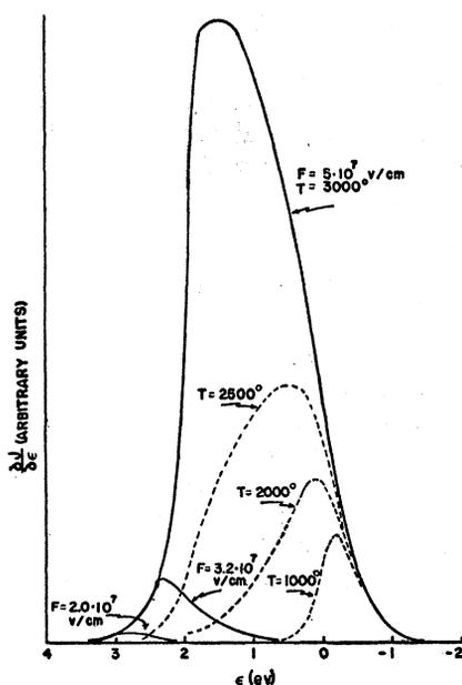
FIG. 3. Energy distributions for emitted electrons with  $\phi=4.5$  eV and at various fields for a constant temperature  $T=3000^\circ\text{K}$  (solid curves); a constant field of  $5 \times 10^7$  v/cm at various temperatures (dashed curves).
