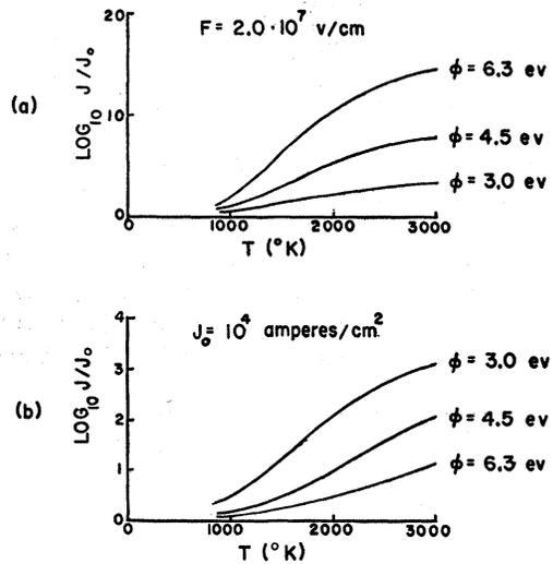
FIG. 5. Graphs showing the dependence of the ratio  $J/J_0$  on temperature  $T$  and work function  $\phi$  at (a) a constant electric field  $F = 2.0 \times 10^7$  v/cm and (b) a constant value for  $J_0 = 10^4$  amp/cm<sup>2</sup>;  $J$  is calculated electron emission current density and  $J_0$  is field current density for  $T = 0^\circ\text{K}$ .
