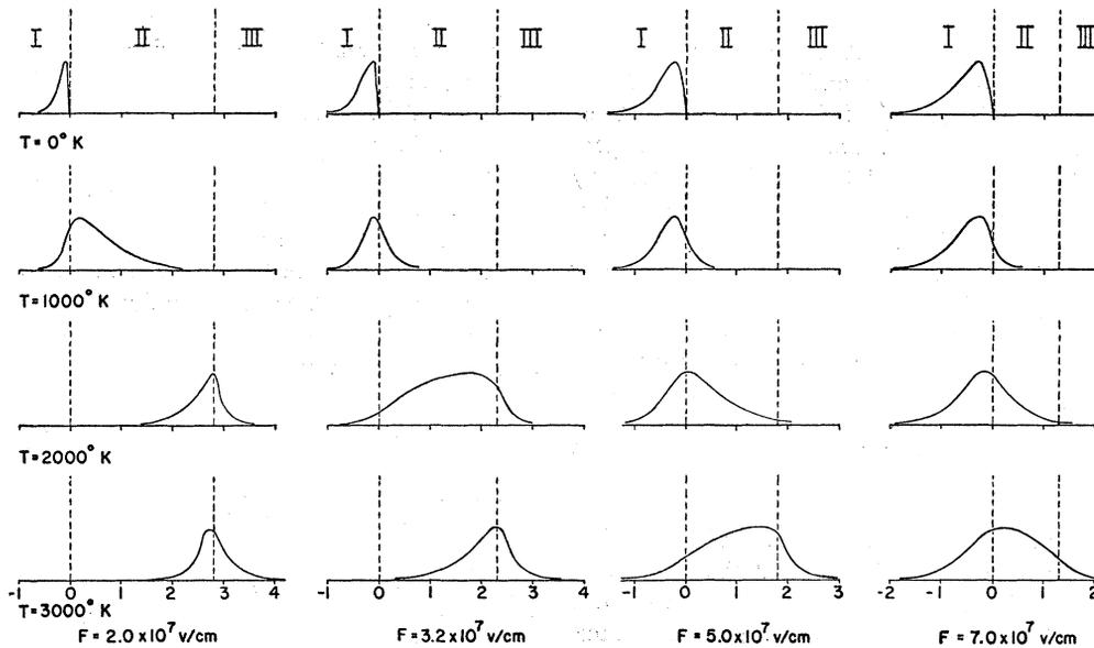
FIG. 2. Theoretical energy distributions for emitted electrons at indicated fields and temperatures, for  $\phi=4.5$  eV, with amplitudes arbitrarily normalized to a common maximum; abscissas  $\epsilon$  in eV relative to the top Fermi level at 0. Regions I, II, and III correspond to those in Fig. 1.
